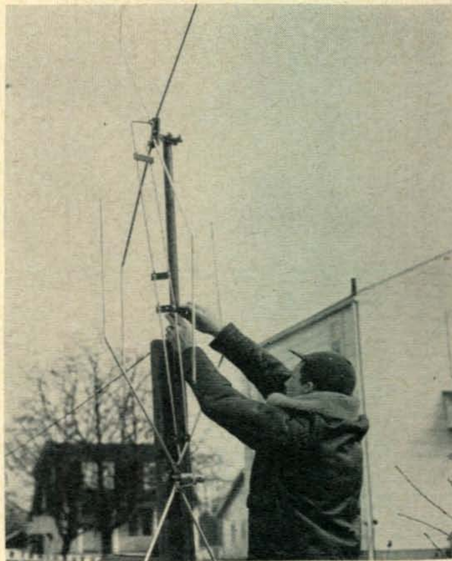
W2SPV puts the finishing touches on his Rocket Quad. A 300-ohm feedline is used. The line was supplied by W2AJG of Saxton Products and is one of their new developments in open wire lines.
